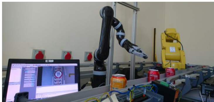
FIGURE 2. Workbench: Kinova robotic arm and Laptop PC with Machine Vision Software
